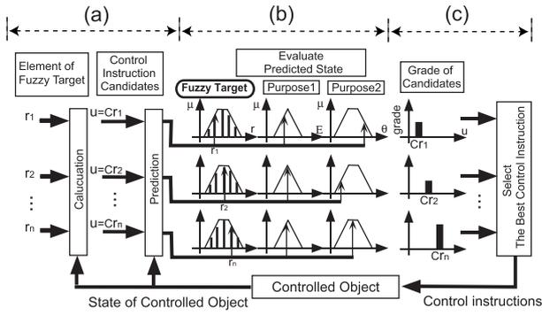
Fig. 3 An intelligent controller based on fuzzy target.
